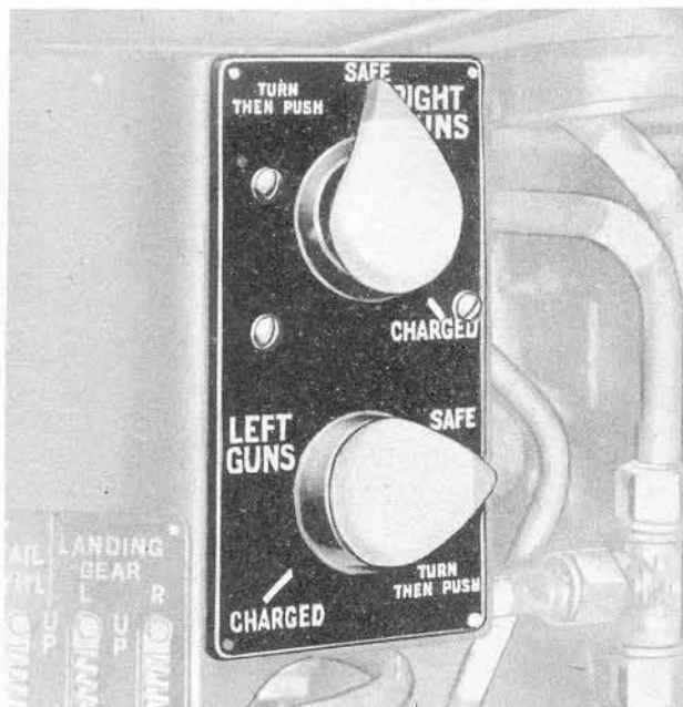
Figure 16—Gun Charging Controls
