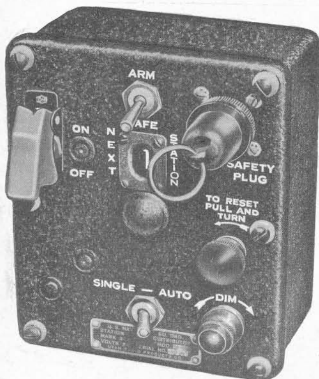
Figure 34—Rocket Station Distributor Box
